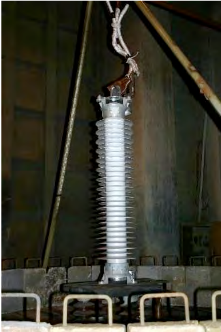
Figure 2. Test sample mounted in test chamber
