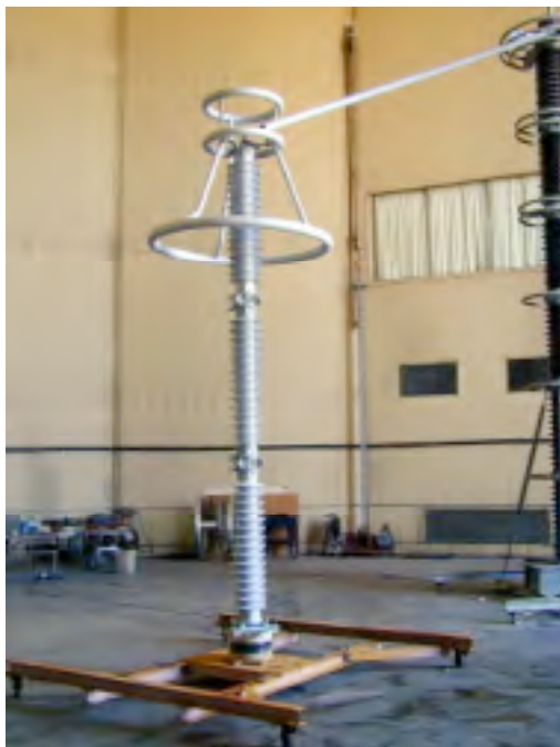
Figure 1. 312 kV rated arrester
