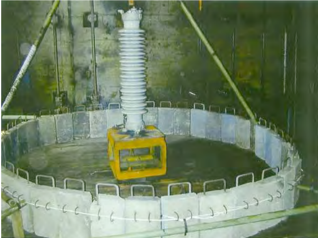
Figure 2. Test sample mounted in test chamber
