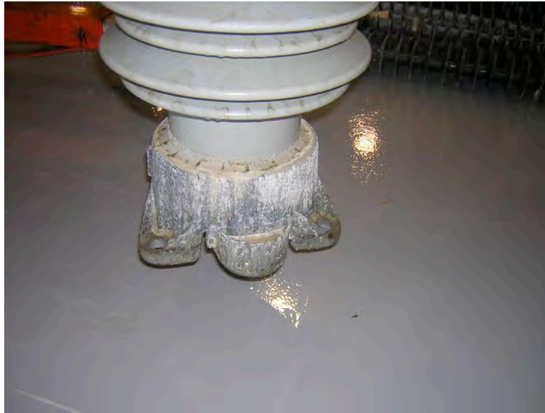
Figure 4. Bottom end of test sample at end of salt mist portion of test
