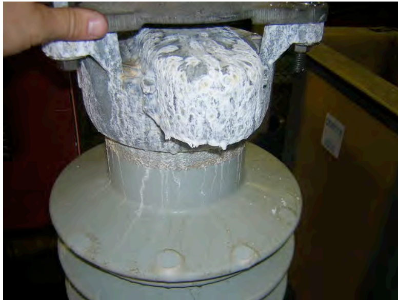
Figure 3. Top end of test sample at end of salt mist portion of test
