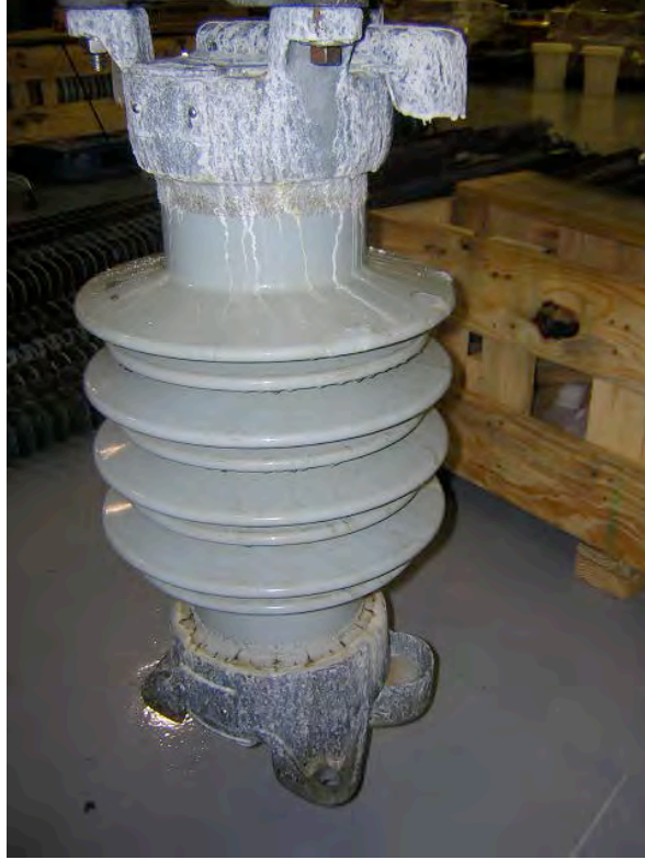
Figure 2. Test sample at end of salt mist portion of test
