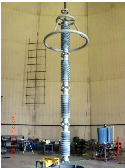
Figure 1. Arrester ready for test
