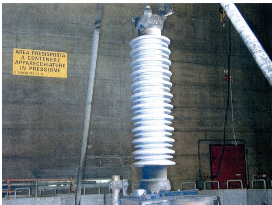
Figure 10. Condition of sample after Oscillograms for 25000A test
