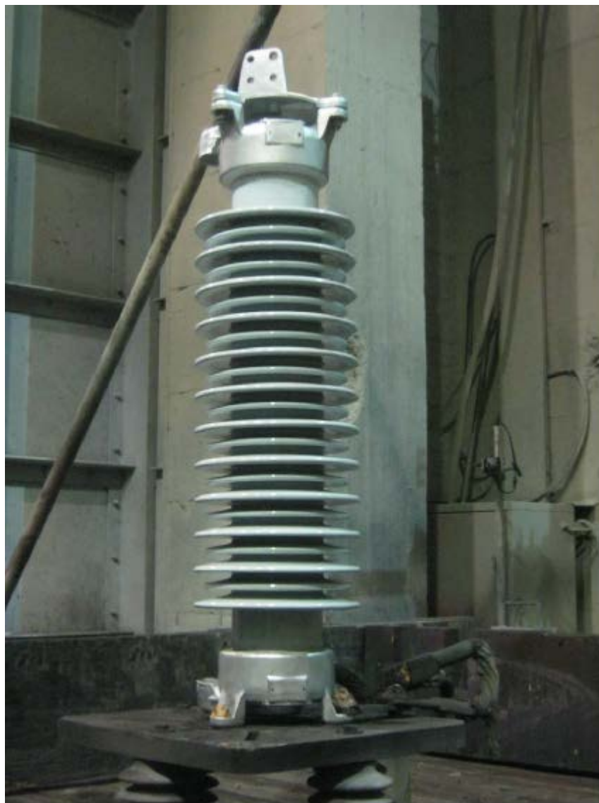
Figure 2. Test sample mounted in test chamber
