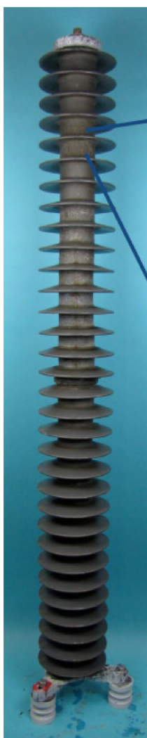
Figure 1 - Arrester condition after 1000 hour salt fog test
