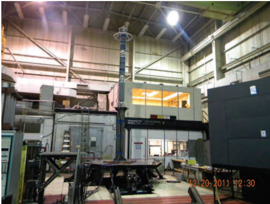
Figure 1. Type MH4, IEC Class 4, Surge Arrester mounted on the Tri-axial Table
