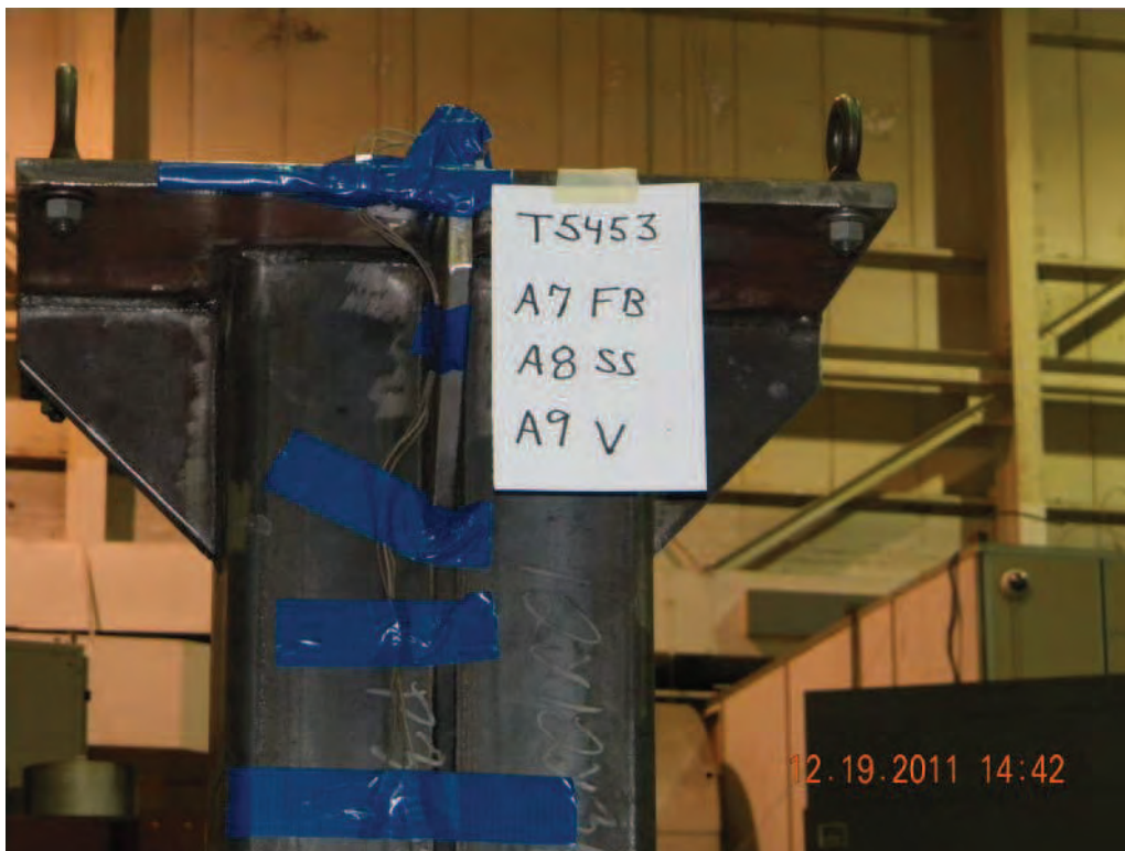
Figure 4. Accelerometer Locations A7, A8 and A9
