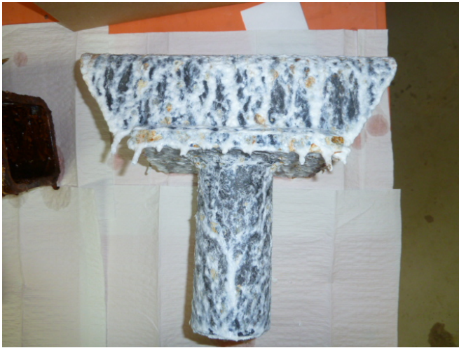
Hot-Dip Galvanized (1040 Hours)
