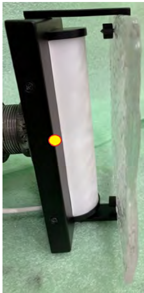
Yellow dot indicates goniometer center, vertically and position along the photometer axis
