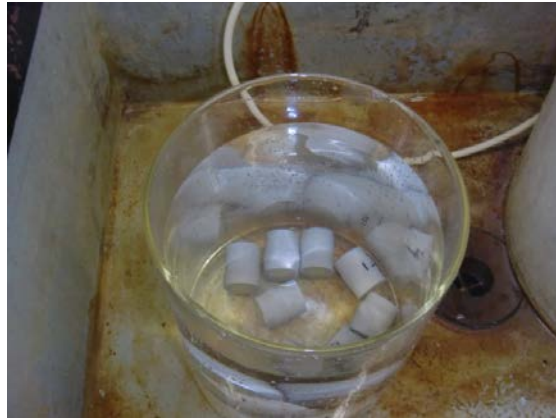
Picture 3: Samples are cooled for 15 minutes in tap water before electrical testing
