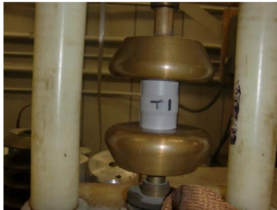
Picture 4: Samples are dried with filter paper and placed between electrodes
