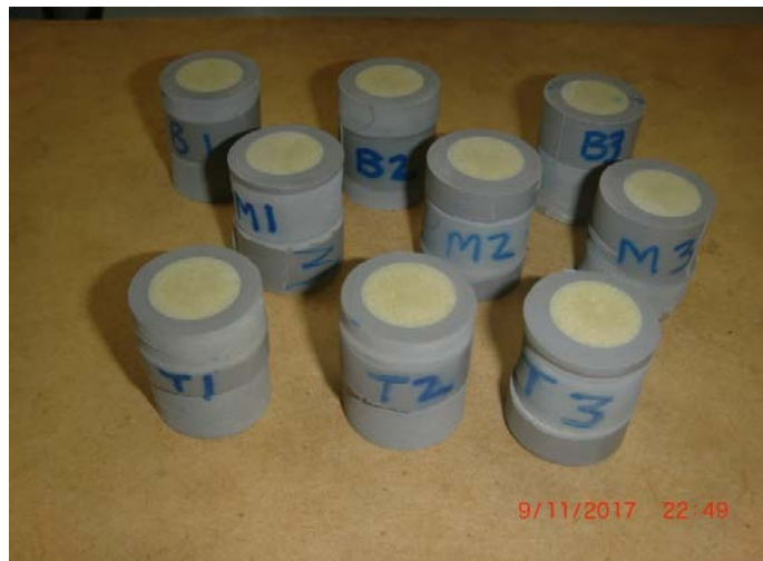
Picture 5: Samples sectioned from the top, middle, and bottom of insulator sample
