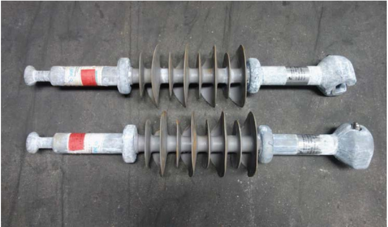
Picture 2 – Condition after 1000 hours Tracking and Erosion
