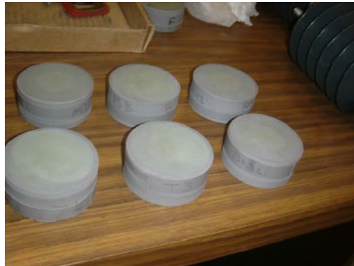
Picture 1: Samples cut from the top, middle, and bottom of sample insulator
