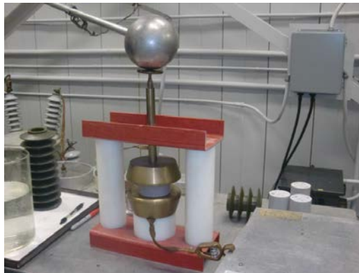
Picture 2: Sample dried with filter paper and placed between the electrodes
