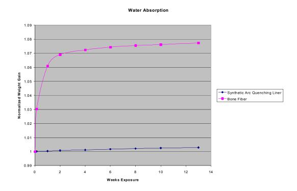
**Conclusions:** The fuse tubes lined with synthetic arc quenching material are virtually immune to moisture absorption.
